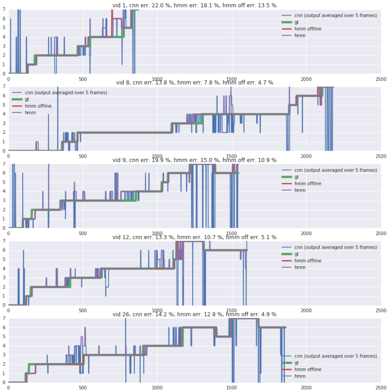
Figure 1. Comparison of our temporal models predictions on the validation set. In blue, our ResNet200 Fine-tuned with average smoothing over 5 frames. In red, the offline predictions of an HMM trained of top of the latter model predictions. In mauve, the online predictions. In green, the ground truth label.
